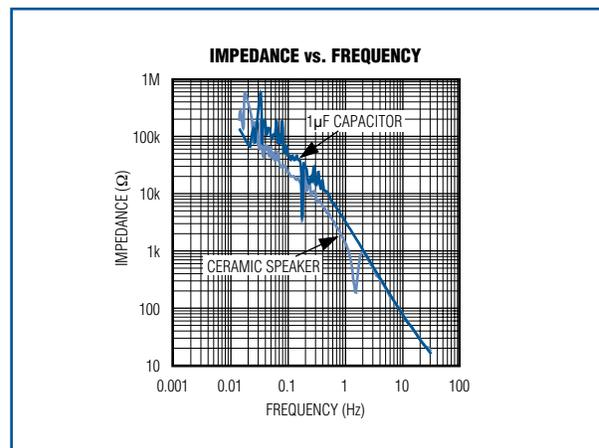
Figure 2. The impedance versus frequency of a ceramic speaker is very similar to that of a  $1\mu\text{F}$  capacitor.
